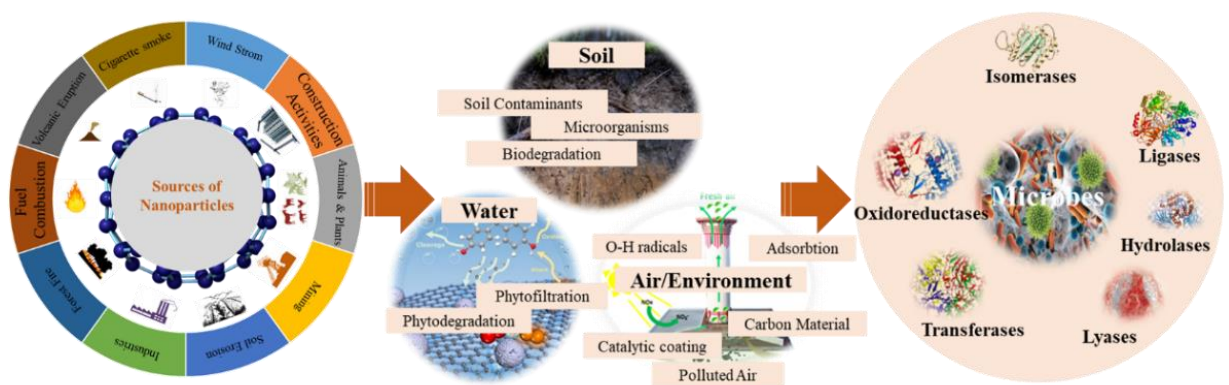
Figure 3. Role of nanoparticles in environmental clean-up. The figure depicts the sources of nanoparticles and their mechanisms of action in remediation of contaminated soil, water, and air/environment. It outlines the enzymatic processes involved and the effectiveness of various nanoparticles in sequestering or degrading heavy metal pollutants. These extended captions provide a comprehensive description of each figure, ensuring that readers can fully understand the implications and contexts of the visual data presented.
